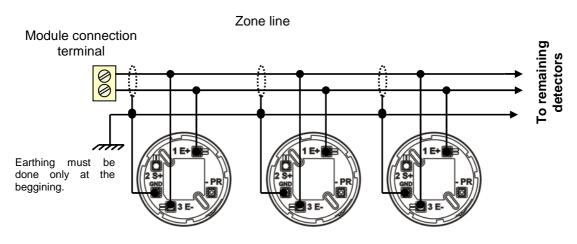
Wiring can be run in free architecture and polarity is not sensitive. Recommended section wiring thickness is  $1.5~\text{mm}^2$
